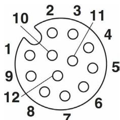
Pinout general purpose input output
