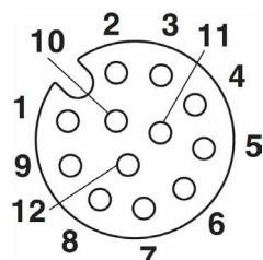
Pinout general purpose input output
